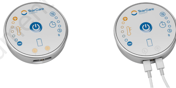
Figure 3. Status of SmartLids: No SmartLids plugged in (Left); Both SmartLids plugged in and functional (Right)
